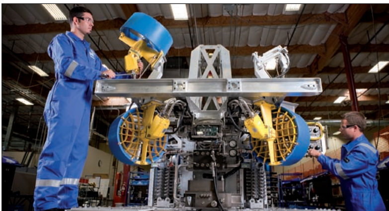
LEFT: Schilling ROV assembly technicians installing a ROV thruster and DTS control units.
