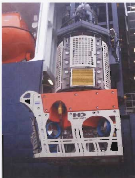
Schilling Robotics' HD Vehicle Being Recovered from Work in the Gulf of Mexico.
