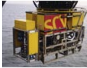
Rear-Mounted IHPU tool-skid (photo: Acergy)
