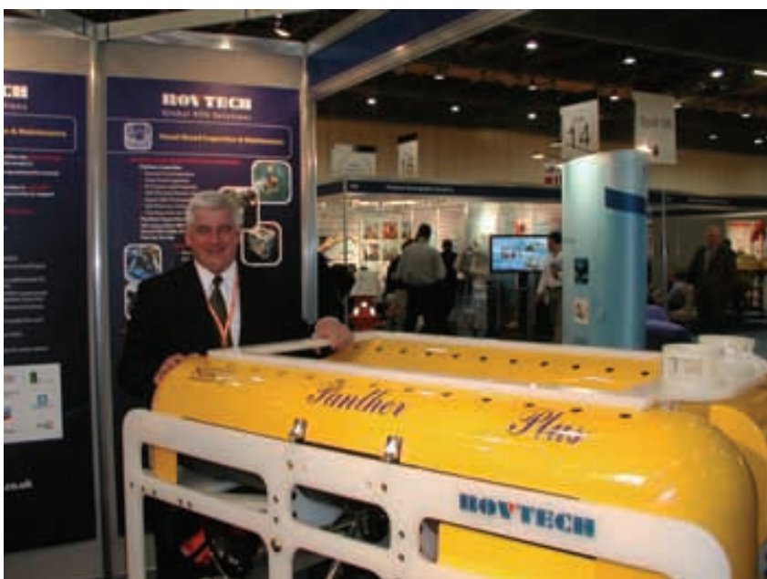
Ian Harvey, Tooling Manager for ROVTECH stands behind their SeaEye Panther Plus Electric Work Class ROV. (Photo Credit: Maggie L. Merrill)
