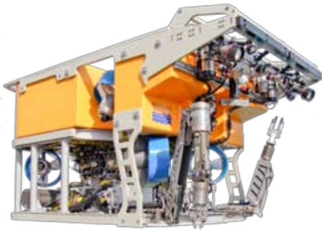
The RIGMASTER is paired with an ORION manipulator arm on the Schilling QUEST™ ROV.
